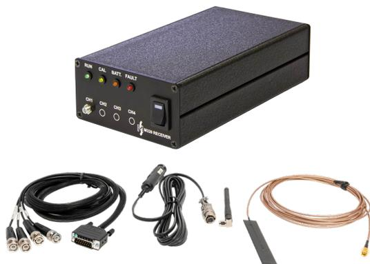
Each Telemetry Receiver picks-up the digital RF signal transmission from its paired Telemetry Transmitter, filters the signal, and provides a  $\pm 10V$  analog output signal. Each receiver has two receiving antenna inputs for more reliable reception, 4 indicator LEDs, and a user adjustable potentiometer for offset adjustment.
